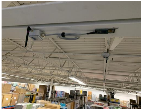
Left: Resensys wireless strain gauge ( SenSpot™ ) used to monitor strain, stress, and deflection on joists; Right: a wireless SenSpot installed at a joist
