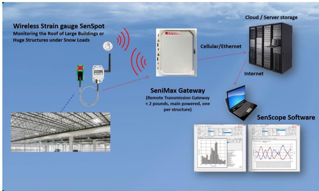
Illustration of Resensys SHM diagram based on SenSpot™ sensors for monitoring the roof of large building or huge structures under snow loads
