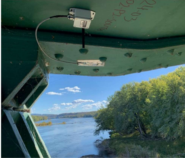
Resensys Wireless Strain SenSpot™ sensor in girder for FEM model verification and validation
