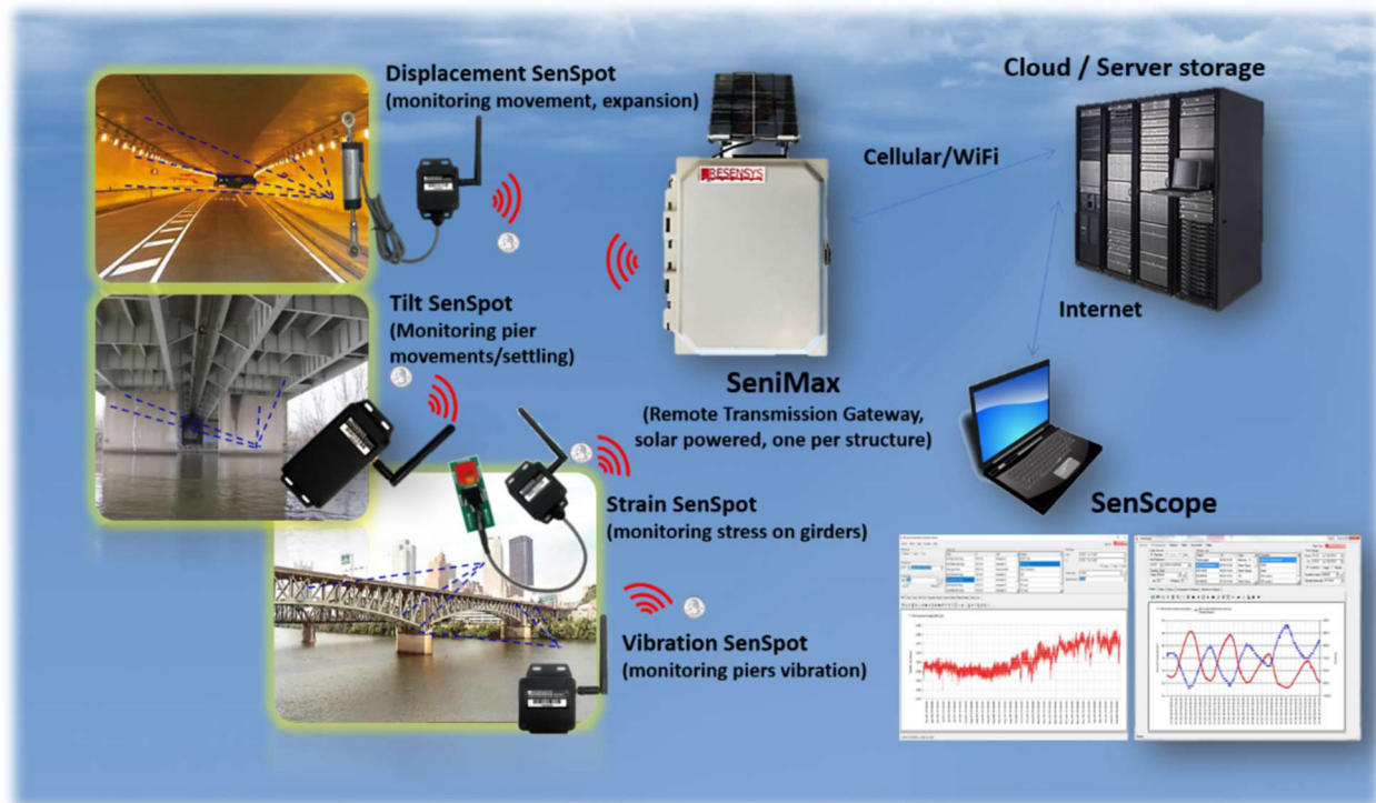
Illustration of Resensys SHM based on SenSpot™ sensors for finite element method (FEM) model verification and validation
