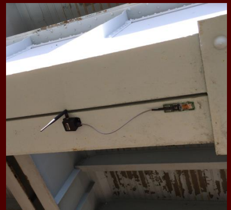
Resensys SenSpot™ sensors monitor 6000 -foot Gold Star Memorial Bridge (I-95 over Thomas River, Connecticut)
