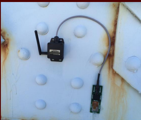
Resensys SenSpot™ sensors monitor 6000 -foot Gold Star Memorial Bridge (I-95 over Thomas River, Connecticut)
