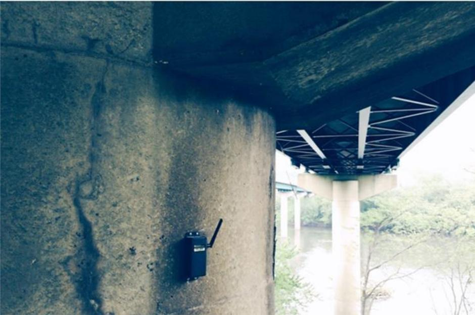
A scour critical I-81 bridge across the Potomac River is monitored using Resensys Wireless Tilt Meters.
