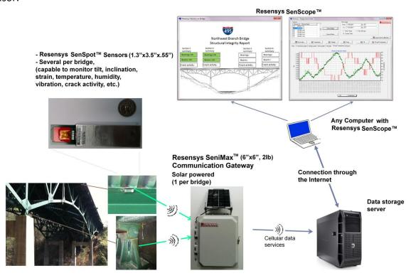
As an example, illustrated in the above picture, Resensys system is used for a bridge structural health monitoring. The system consists of three main components:
